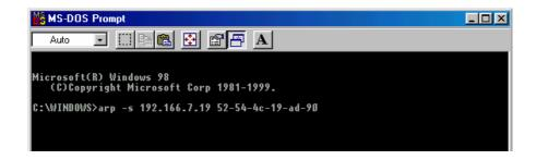
6. This is an example. At the MS-DOS Prompt type: arp -s 192.166.7.19 52-54-4c-19-ad-90. Then hit enter. The first string is the IP Address; the second string is the MAC Address (which can be found on the front of the iSwitch).
